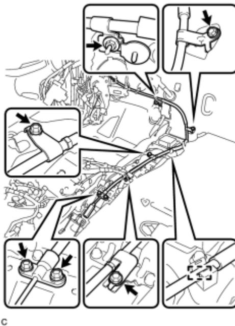
(a) Remove the 5 bolts and nut, and separate the No. 1 parking brake cable assembly.
